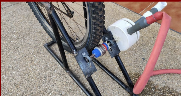
Fig.11a – The shaft connected to the bike wheel
