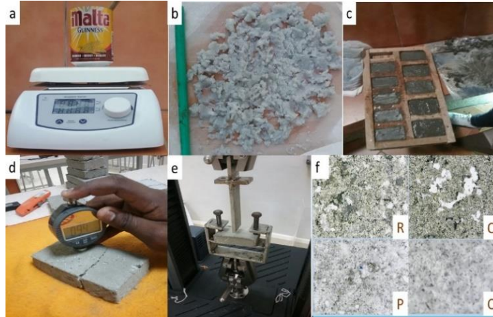
Figure 1. Procedure (a) Melting of plastics, (b) Drying of the plastic granules, (c) Molding of blocks, (d) Testing Hardness, (f) Microscopic surface analysis of different samples.
