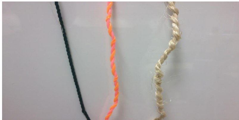
Figure 1. A picture of the three samples: nylon(deep green), rubber(orange), and sisal (white).
