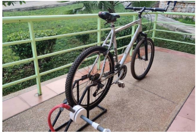
Fig.11b – Complete bike water pump
