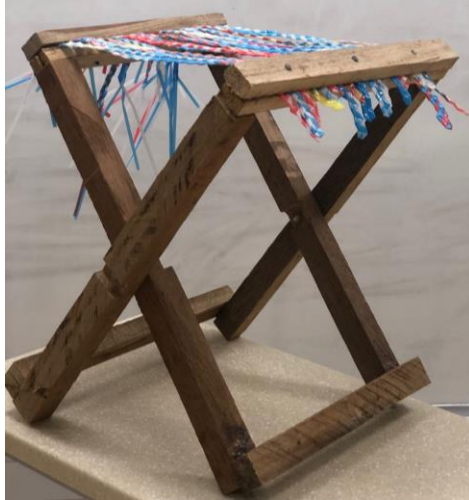
Fig. 5 Resulting foldable wooden stool with seating area made out of plastic straw woven in a rustic plait.
