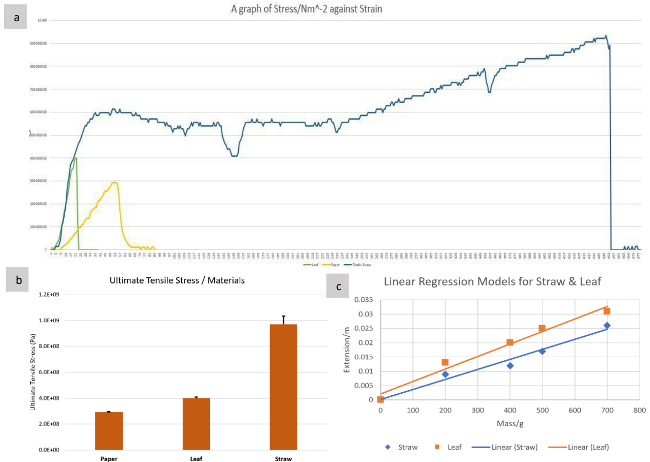
Fig. 3 (a) Tensile stress against strain graph. The blue curve representing straw, green representing Brahea Edulis leaf strip and yellow representing double-layered paper strip. (b) Bar graph of mean ultimate tensile stress of each material. Error bars represent standard deviation. (c) Graph of mass against extension with lines of best fit plotted for each material. The orange line represents the Brahea Edulis leaf strip, and the blue line represents the plastic straw.
